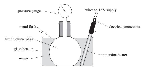
(a) The student used the immersion heater to heat the water in the beaker.
