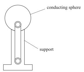
The conducting sphere of a Van de Graaff generator has a radius of 22.5 cm.
