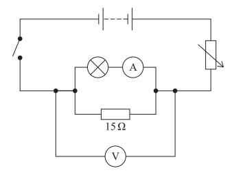
(a) The student adjusted the variable resistor and recorded corresponding values of current and potential difference for the lamp.
