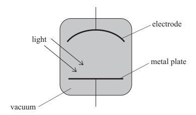
Light incident on the metal plate can cause the photoelectric effect.
