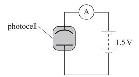
Photoelectrons are attracted to the electrode, causing a current in the circuit.
