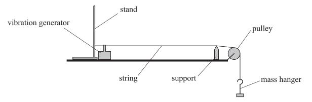
The student adjusted the frequency of the vibration generator until a standing wave formed on the string, as shown below.
