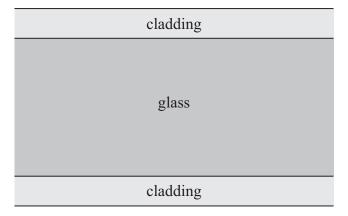
The transparent material has a lower refractive index than the glass of the optical fibre.
