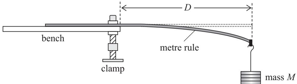
The student displaced the mass vertically and allowed it to oscillate.
