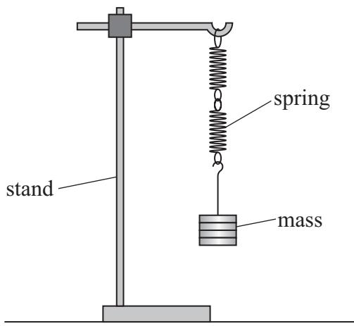
The student displaced the mass downwards and allowed the mass to oscillate.
