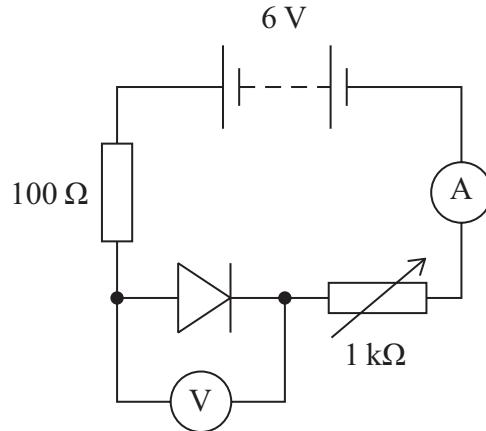
He used the ammeter to measure the current as he varied the temperature of the diode.
