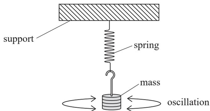
When the mass is displaced through a small angle, the mass performs rotational oscillations about a vertical axis through the spring.
