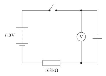
The student closed the switch to charge the capacitor and started a stopwatch. She recorded the voltmeter reading V every  $10 \, \mathrm{s}$  as the capacitor charged.
