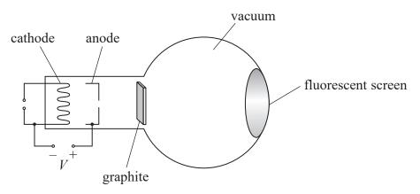
A potential difference V was applied between the cathode and the anode to produce the beam of electrons.
