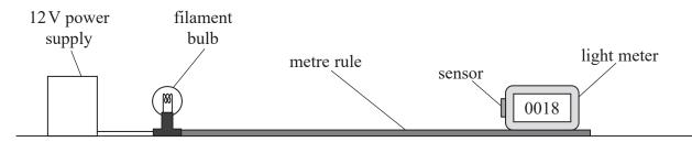
The student used a metre rule to measure the distance d between the filament of the bulb and the sensor on the light meter.
