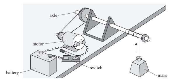
(a) The motor was connected in a circuit including a battery and a switch.
