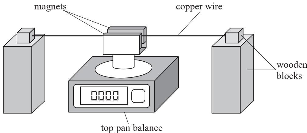
The student connected the copper wire to a circuit which included a power supply with a fixed potential difference. The maximum current from the power supply was 5 A.
