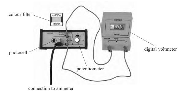
He used a source of white light and colour filters to shine different wavelengths  $\lambda$  of light onto the photocell.
