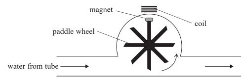
As water flowed through the device the paddle wheel rotated, making the magnet move past the coil.
