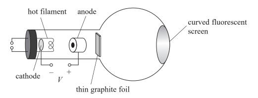
The potential difference, V, accelerates electrons from the hot filament towards the thin graphite foil.
