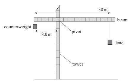
(i) Explain how the counterweight needs to move when the load is moved away from the tower.
