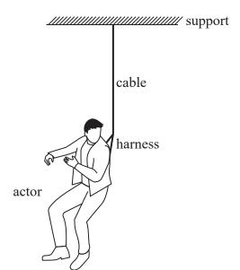
(a) The force on the cable must not cause the material of the cable to reach its yield point.
