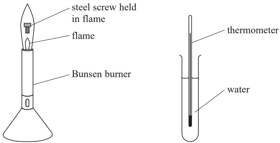
The student held the steel screw in the flame and then cooled it in a test tube of water.
