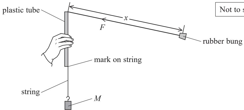
The rubber bung with mass  $m$  was rotated around the plastic tube at a constant angular velocity  $\omega$ . The part of the string between the rubber bung and the plastic tube was almost horizontal.
