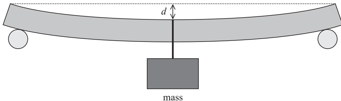
She measured the vertical distance  $d$  moved by the middle of the plastic beam and repeated this measurement for increasing values of  $F$ .
