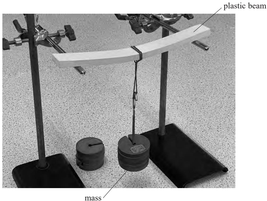
The beam bent downwards as shown.
