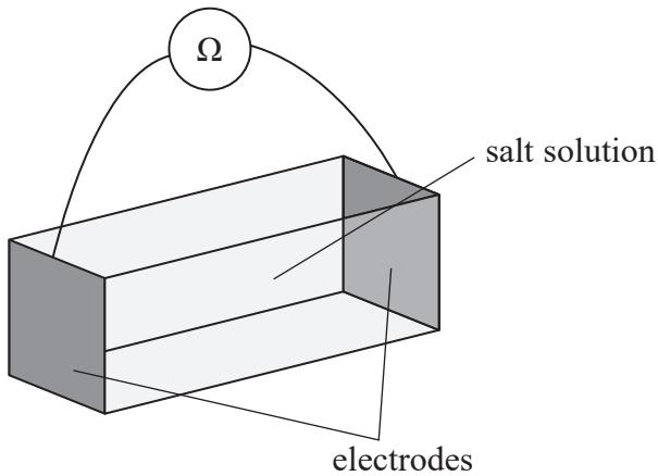
After measuring the resistance  $R$  of the salt solution with the ohmmeter, she calculated the resistivity  $\rho$  of the salt solution.
