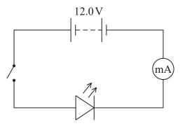
The LED emits light of wavelength of 627 nm and may be assumed to be 100% efficient. The battery has negligible internal resistance.
