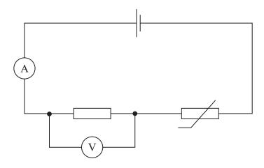
The temperature of the thermistor increases.
