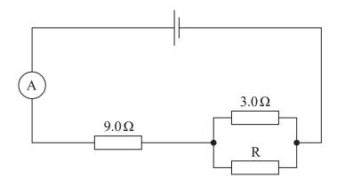
(a) Calculate a value for the resistance of the resistor R.
