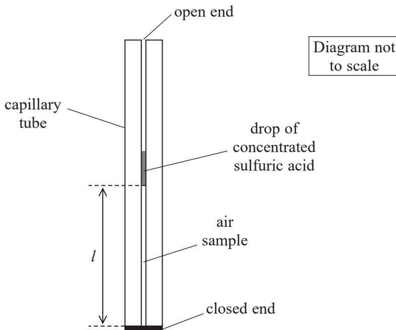
A sample of air is trapped inside the tube between the closed end and the drop of concentrated sulfuric acid.
