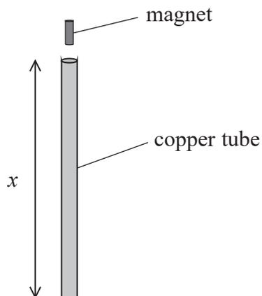
The student dropped the magnet into the copper tube and measured the time  $t$  for the magnet to reach the bottom of the tube.
