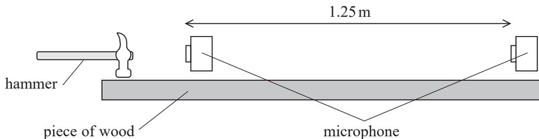
The microphones were connected to a 2-beam oscilloscope. The student hit the wood with a metal hammer producing a sharp sound that travelled through the air. The oscilloscope traces produced by the microphones and the time per division dial are shown.
