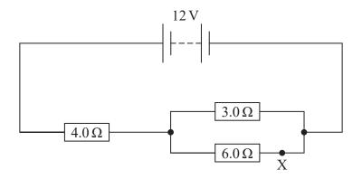
(a) Calculate the number of electrons passing point X each second.
