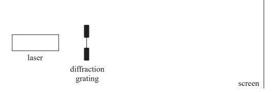
When the laser is switched on, a series of bright dots is seen on the screen.
