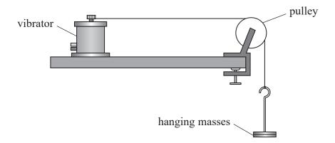
The frequency f of the vibrator was adjusted until a stationary wave was formed with a node at each end. This was repeated for various stationary waves on the string. A metre rule was used to measure the distance d between adjacent nodes on the string.
