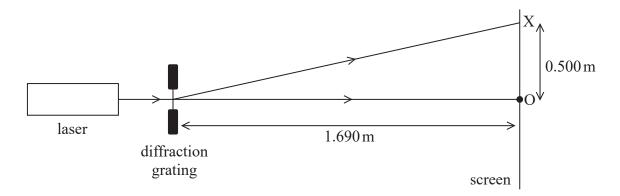
Determine the wavelength of the light from the laser.
