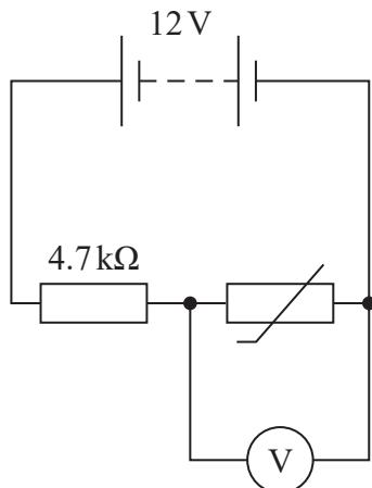
She heated the thermistor to 100 °C and measured the potential difference  $V$  across it. She decreased the temperature  $\theta$  and recorded further measurements of  $V$  and  $\theta$  until the temperature reached 10 °C.
