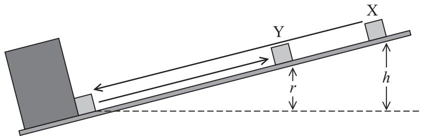
The student measured heights  $h$  and  $r$ . He then repeated the experiment using several different starting positions.
