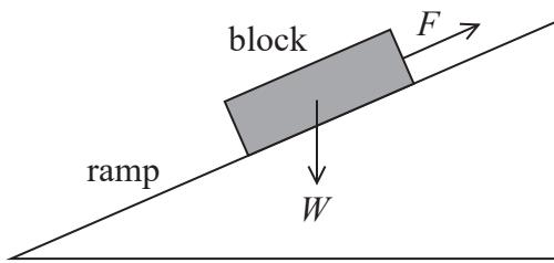
A triangle of forces can be used to determine the magnitude and direction of the normal contact force  $N$  acting on the block.
