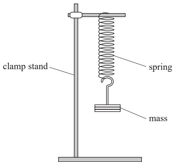
She set the mass into vertical oscillations by displacing it a small distance from its equilibrium position. The spring obeys Hooke's law.
