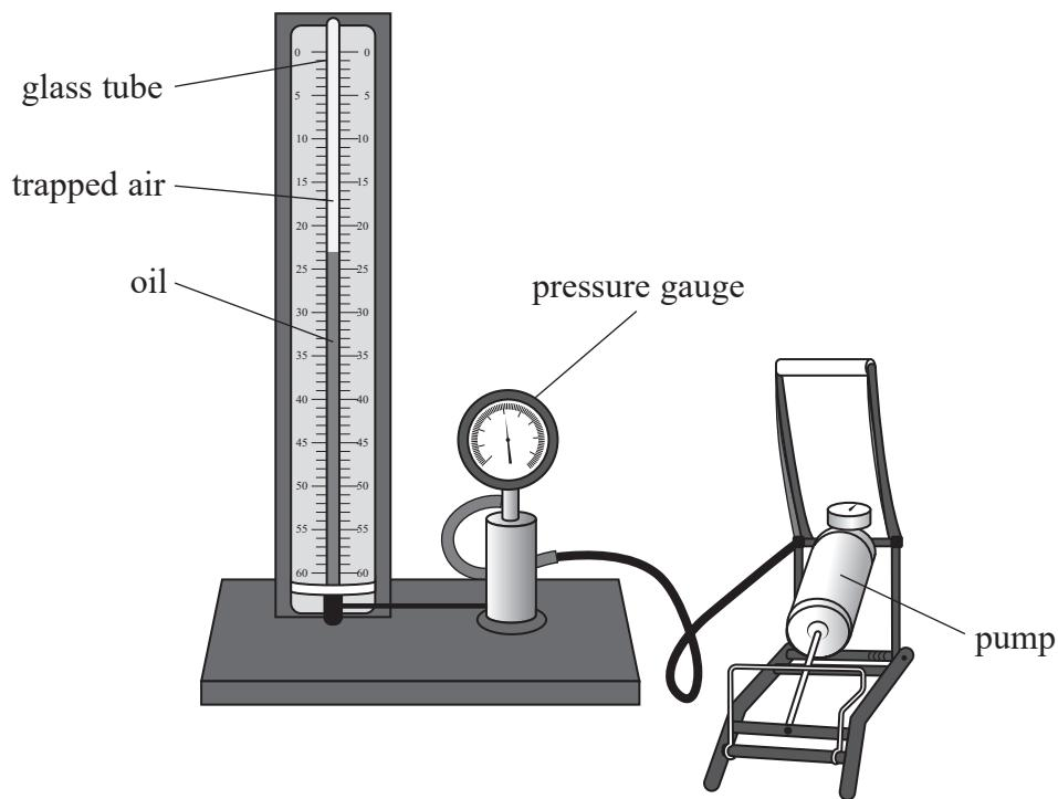
Air is trapped in a glass tube of uniform cross-sectional area. A pump forces oil into the base of the glass tube. This forces the air into a smaller volume. The pressure of the trapped air is displayed on the pressure gauge.
