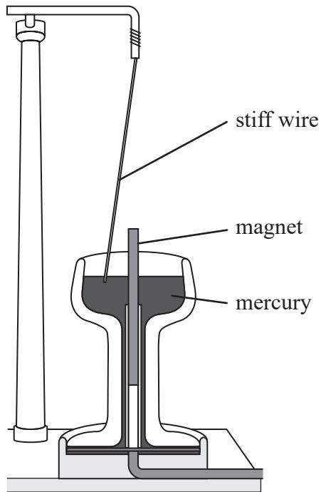
The stiff wire was suspended freely from a stand. The mercury completed an electrical circuit, which included the wire. When there was a current in the wire, the wire moved around the magnet.
