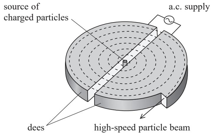
\*(a) Explain the role of electric and magnetic fields in the production of high-speed charged particles by a cyclotron.
