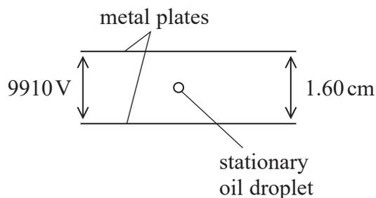
Calculate the charge on the oil droplet.
