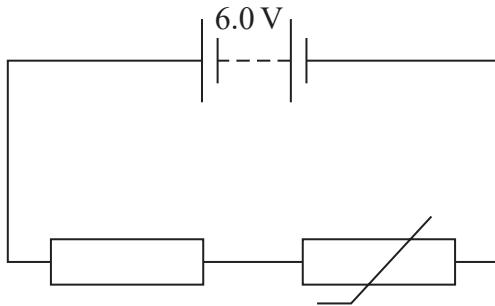
The thermistor acts as a temperature sensor. When the temperature reaches  $0^\circ\text{C}$ , the potential difference across the thermistor becomes 5.0 V, which switches on a heater.
