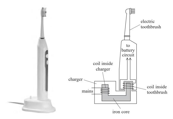
The charger contains a coil wrapped around an iron core. The coil is plugged into the mains supply. The toothbrush also contains a coil that sits around the iron core when the toothbrush is placed on the charger.
