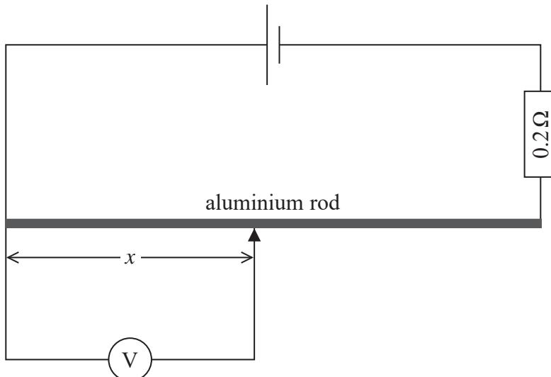
The voltmeter was connected to the aluminium rod to give three different values of  $x$ . The values of  $x$  and potential difference (p.d.)  $V$  were recorded.
