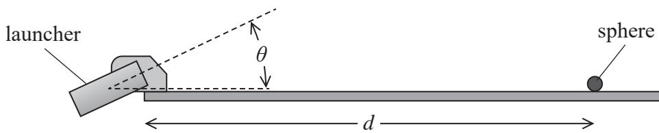
The student measured the horizontal distance  $d$  travelled by the sphere for different launch angles  $\theta$ .
