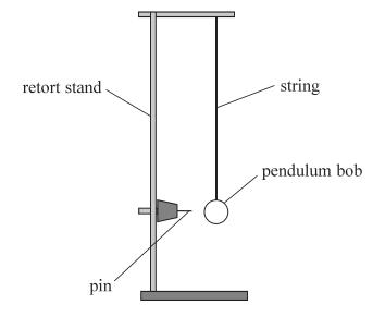
The pendulum performs simple harmonic motion, hence T is given by the equation
