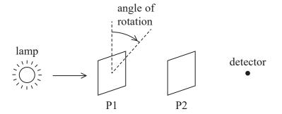
The filters initially have their planes of polarisation perpendicular to each other.
