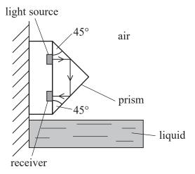
When the liquid is below the level of the prism the light totally internally reflects to the receiver as shown.
