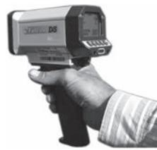
The speed gun emits pulses of infrared radiation every 0.250 s. The pulses are reflected by a moving car and then detected by the speed gun, which calculates and displays the speed of the car.
