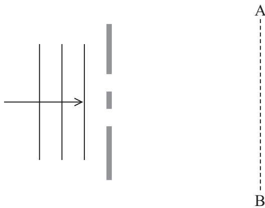
A microwave detector was moved along the line AB. Variations in intensity were detected.
