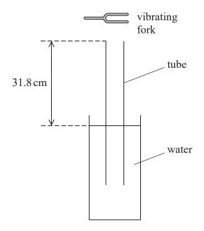
A vibrating fork is held above the other end and the tube is moved slowly upwards in the water. At a particular position the sound is loudest. When this occurs, there is one node and one antinode. The node is at the surface of the water and the antinode is at the top of the tube.
