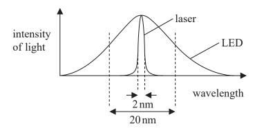
Light of different wavelengths will travel at different speeds along the fibre. Use the graph to compare lasers and LEDs as light sources for a communication system.
